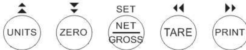
4. After setting the exact value, press the NET/GROSS key to save the ID Number value. The display will show "**SET**" momentarily, and then revert back up to A8.
