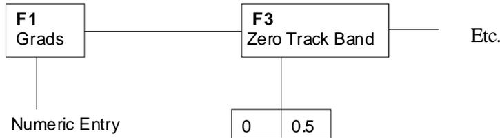
1. To move to a new heading, use the TARE (left) or PRINT (right) key to move right or left in the Menu.
